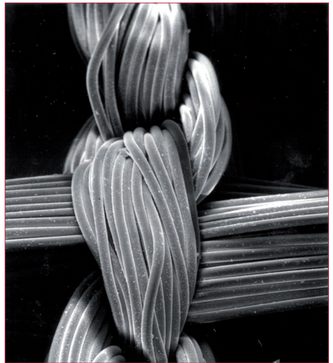
Figure 1b. Microscopic view of a typical paraffin gauze showing absence of ordered fibres.
