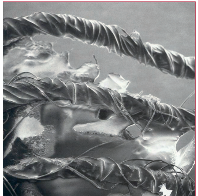
Figure 1b. Microscopic view of a typical paraffin gauze showing absence of ordered fibres.
